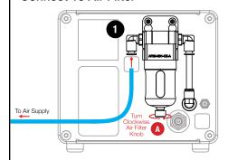
Power off engraving system and air supply. Insert hose from air supply to filter fitting marked "Air Input" (see 1) until the hose stops and is secure.
