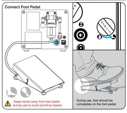
Power on air supply and GRS® Air System to check for leaks and improper connections; air should not escape through any hose or fitting. If air leaks, power off system and air supply. Locate leaks and correct any improper connections. To disconnect from a push-to-connect fitting, press in on the front of the fitting while
