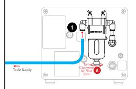
Power off engraving system and air supply. Insert hose from air supply to filter fitting marked "Air Input" (see 1) until the hose stops and is secure.
