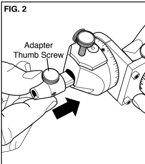
To mount the adapter, completely open the Dual Angle Fixture jaws. Insert the adapter with its longest edge lying across the bottom of the fixture jaws (**FIG. 2**).
