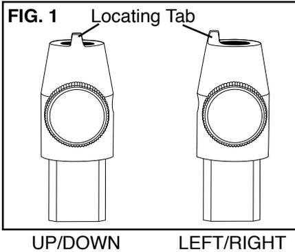
Select which adapter to use according to personal preference and work style. One adapter will allow the QC Tool Holder locating tab to be either UP or DOWN. The other adapter will allow the locating tab to be either in the LEFT or RIGHT position (**FIG. 1**).
