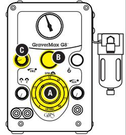
Hold the handpiece you have selected to use vertically, tool holder end up, next to your ear. Without depressing the foot throttle or palm control, **SLOWLY** increase the air pressure until the handpiece begins to buzz. Continue to increase the air pressure until the handpiece vibrates and knocks. Slowly add air pressure until the knocking stops. This is the perfect air pressure for each handpiece. Now you are free to move the SPM (strokes per minute) dial to whatever setting desired.
