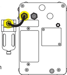
Find the black hose 139mm (5 1/2"). Connect one end to the **air input quick connect fitting** on the back of the machine and the other end to the straight **quick connect fitting**.
