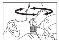
Hold to your ear and turn knob until you hear it stop stroking. You can feel it stop too. Turn knob in about 1/2 turn and tighten the locking ring.
