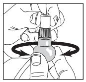
Unscrew knob until the handpiece strokes without using throttle.
