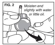
outside end of the hose next to the brass fitting and pull the hose back (FIG. 2) into the knob until you see the tip of the brass fitting protrude through the side of the knob. This must be an airtight fit, so you will have to pull somewhat hard (a few pounds, at least).
