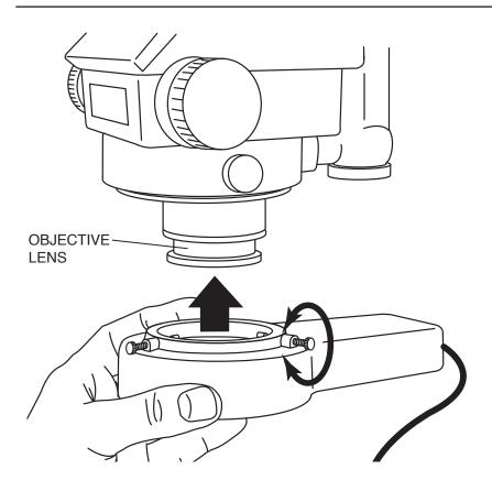
First, turn the three thumb screws out as far as they will go. Position the light over the objective lens. Turn the thumb screws in - equally - until the light fixture is held securely. Do not overtighten. Plug the light in and turn it on with the switch on the back.
