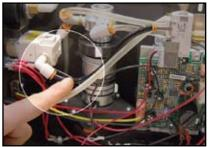
Connect longer black hose to the solenoid and the "SUP" side of the regulator. Press the fitting downward to take up any slack in the hose.
