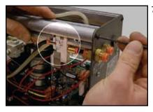
7. Note how the rail gap fits around the solenoid valve. Install the modified top rail (do not forget to put the 4 nuts in the rail). Before replacing the panels, check to make sure the valve works with air applied.
