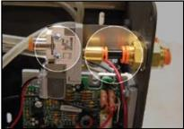
Install valve by connecting the short black hose to the AIR INLET port. Install screws, nuts to the inside of the bracket.
