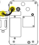
Find the black hose 139mm (5 1/2"). Connect one end to the **air input quick connect fitting** on the back of the machine and the other end to the straight **quick connect fitting**.
