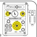
quick connect fitting you are using. Set the **stroke per minute** (A) to 2300. Set the main air regulator knob (B) to 0.1 ~ 0.4 BAR (2~5 PSI). Close the bias control valve (C).
