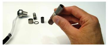
Completely disassemble the handpiece. The two main components you will be servicing are the barrel, which has a precision bore for the piston, and the piston itself.
