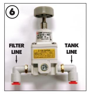
Note the arrow on the regulator. It shows the correct air flow direction. The incoming line from the filter goes on the "IN" side and the line from the regulator to the tank goes on the "OUTPUT" side as seen on the back of the regulator housing.
