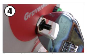
Use a wrench to remove the regulator mounting nut
