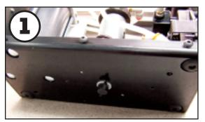
Before beginning this replacement, disconnect the air and electrical supply lines and install the motor mount locking screw.
