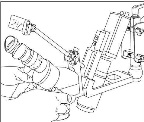
Transfer the headrest from the old microscope holder assembly (F) and tighten gently.
