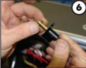
Make sure the exterior o-ring (#002-333) is still on the valve stem and next to the plastic valve body, then slip the smaller washer over the brass valve stem.
