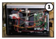
As you look at the front of the machine, remove the side cover on the right side. This is done by using a 1/8" hex key and removing the 2 button head screws at the top of the side cover and loosen the 3 button head screws at the bottom of the side cover. Gently lift the side cover off. (*Note: You may have to loosen the button head screws on the back panel to relax the cover to allow for easier removal.*)
