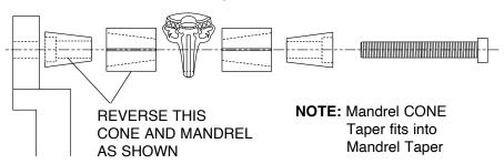
To hold large / wide rings, use TWO of the SAME SIZE mandrels and TWO mandrel cones. Insert the long bolt through the first mandrel cone and place cone into the tapered end of the mandrel selected. Then reverse the second mandrel and place on bolt. Slide the second cone into that mandrel so that the taper angles match. (See illustration above) Position ring on the selected mandrel. Tighten the socket head screw into the Ring Post with the supplied wrench until the ring is snug.
