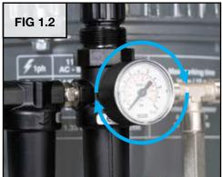
Install the Air Pressure Gauge by threading the gauge into the fitting on the Regulator Air Filter as shown.
