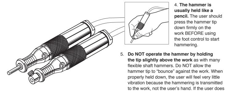
4. The hammer is usually held like a pencil. The user should press the hammer tip down firmly on the work BEFORE using the foot control to start hammering.
